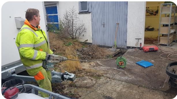
*Drilling holes in the Innovation Garage test site for vapor transport experiments. The trailer on the left belongs to a private consortium, who tested a new groundwater remediation method at the site.*
