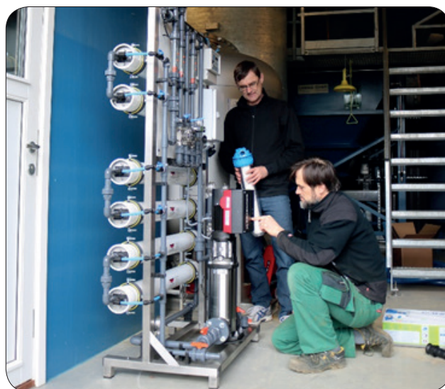
Testing the membrane system at the Stengaarden test site, Foto: Region Zealand and the Capital Region in Denmark.
