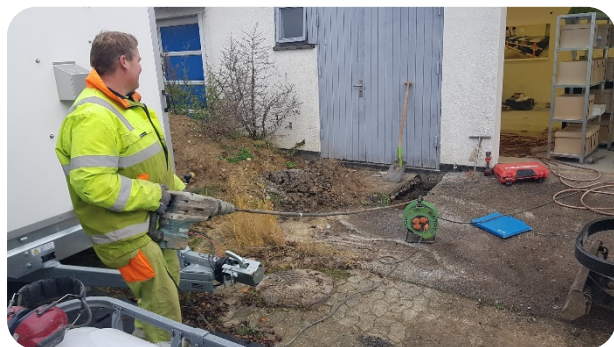
Drilling holes in the Innovation Garage test site for vapor transport experiments. The trailer on the left belongs to a private consortium, who tested a new groundwater remediation method at the site.
